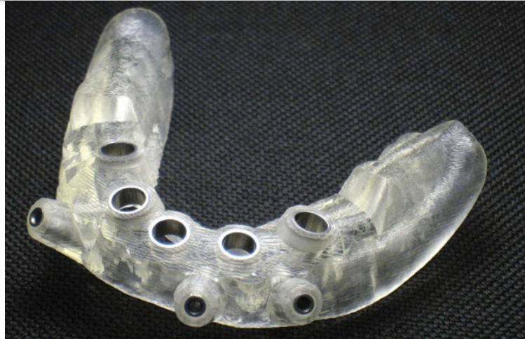
A custom plastic dental drilling guide made on a 3D Systems SLA machine. This aids dentists in drilling holes for inserting tooth implants.
